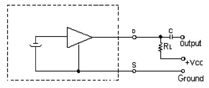
RL=2.2k $\Omega$  (External resistor) +Vcc=4.5V C=1uF
