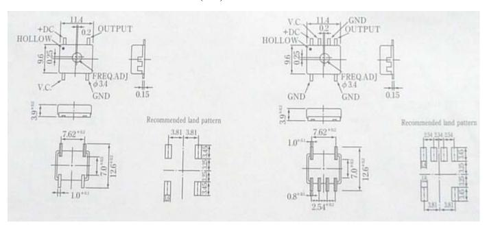
These oscillators are shippen after frequency adjustment at NDK.But if you need totrim frequency by trimmer condenser, please make suer that the driver fits trimmer rotor hole Also do not weigh onto trimmer rotor
