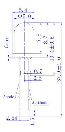
All dimensions in mm, tolerances unless mentioned is  $\pm 0.2$  mm.
