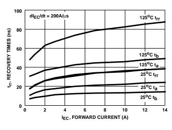
FIGURE 20. RECOVERY TIMES vs FORWARD CURRENT
