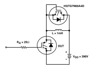
FIGURE 24. INDUCTIVE SWITCHING TEST CIRCUIT
