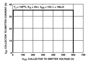
FIGURE 2. MINIMUM SWITCHING SAFE OPERATING AREA
