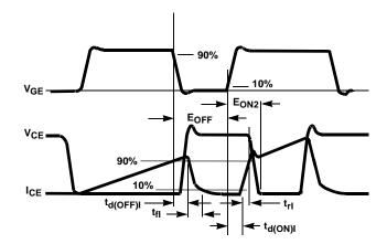
FIGURE 25. SWITCHING TEST WAVEFORMS
