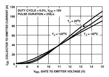
FIGURE 13. TRANSFER CHARACTERISTIC
