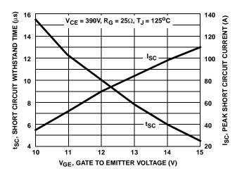
FIGURE 4. SHORT CIRCUIT WITHSTAND TIME
