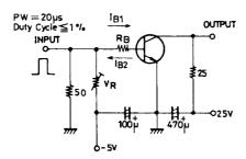
I C=10 I B1=-10 I B2=1A (For PNP, the polarity is reversed.)
