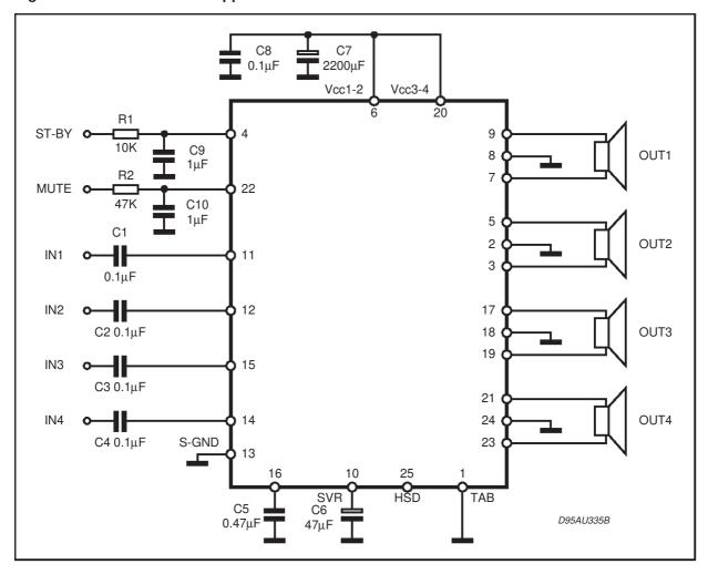
Figure 1: Standard Test and Application Circuit
