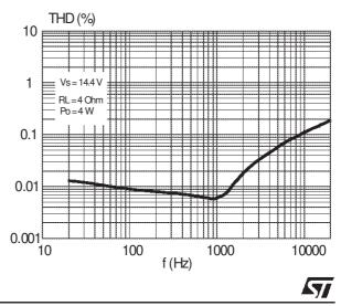
Figure 9. Distortion vs. frequency.
