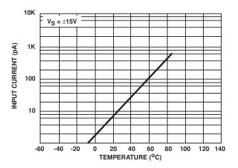
FIGURE 4. INPUT CURRENT vs TEMPERATURE
