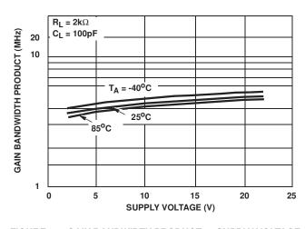
FIGURE 14. GAIN BANDWIDTH PRODUCT vs SUPPLY VOLTAGE
