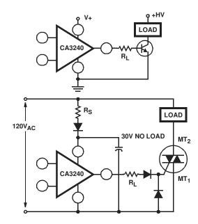
FIGURE 3. METHODS OF UTILIZING THE V<sub>CE (SAT)</sub> SINKING CURRENT CAPABILITY OF THE CA3240 SERIES
