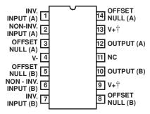
† Pins 9 and 13 internally connected through approximately  $3\Omega$ .
