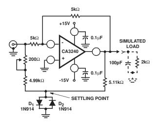
FIGURE 26C. TEST CIRCUIT (INVERTING)
