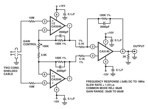
FIGURE 10. PRECISION DIFFERENTIAL AMPLIFIER
