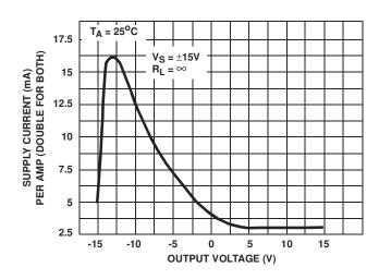
FIGURE 22. SUPPLY CURRENT vs OUTPUT VOLTAGE
