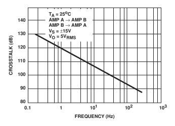
FIGURE 23. CROSSTALK vs FREQUENCY
