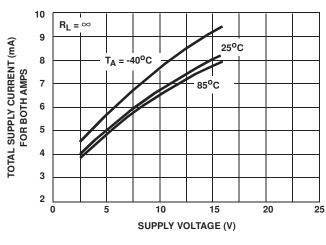
FIGURE 16. QUIESCENT SUPPLY CURRENT vs SUPPLY VOLTAGE
