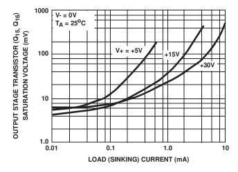
FIGURE 24. VOLTAGE ACROSS OUTPUT TRANSISTORS  $\mathbf{Q}_{15}$  AND  $\mathbf{Q}_{16}$  vs LOAD CURRENT
