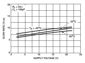
FIGURE 15. SLEW RATE vs SUPPLY VOLTAGE
