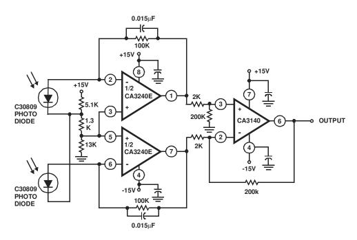
FIGURE 12. DIFFERENTIAL LIGHT DETECTOR
