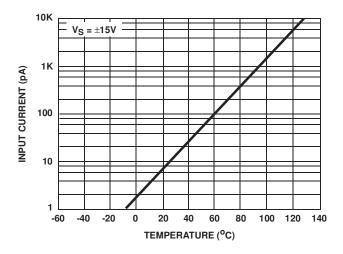
FIGURE 27. INPUT CURRENT vs TEMPERATURE
