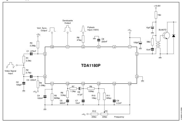
Figure 7: Application Circuit for Small Screen b.w. TV
