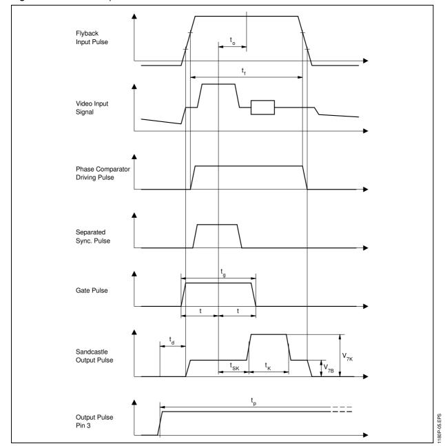
Figure 2: Relation Ship of Main Waveform Phases
