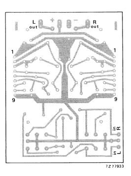
Fig.13 Track side of printed-circuit board used for the circuit of Fig.12; p.c. board dimensions 83 mm  $\times$  65 mm.
