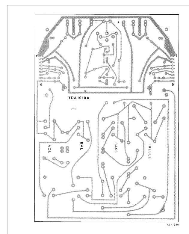
Fig.18 Track side of printed-circuit board used for the circuit of Fig.17 (Fig.16 partly); p.c. board dimensions  $169 \text{ mm} \times 118 \text{ mm}$ .
