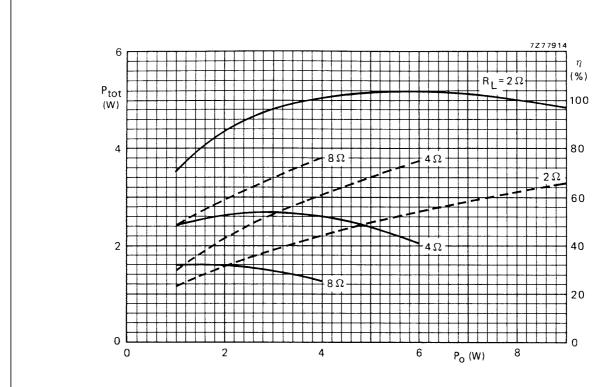
Fig.7 Total power dissipation (solid lines) and the efficiency (dashed lines) of the circuit of Fig.3 as a function of the output power with the load impedance as a parameter (for  $R_L = 2~\Omega$  an external bootstrap resistor of 220  $\Omega$  has been used); typical values.  $V_P = 14.4~V$ ; f = 1~kHz.
