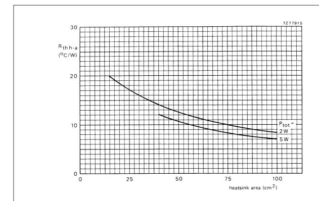
Fig.8 Thermal resistance from heatsink to ambient of a 1,5 mm thick bright aluminium heatsink as a function of the single-sided area of the heatsink with the total power dissipation as a parameter.
