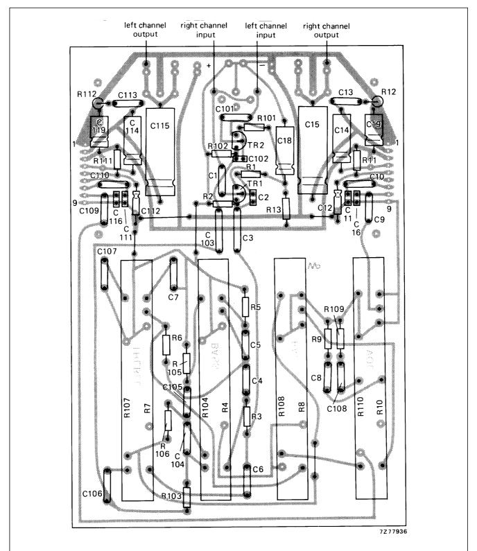
Fig.19 Component side of printed-circuit board showing component layout used for the circuit of Fig.17 (Fig.16 partly).
