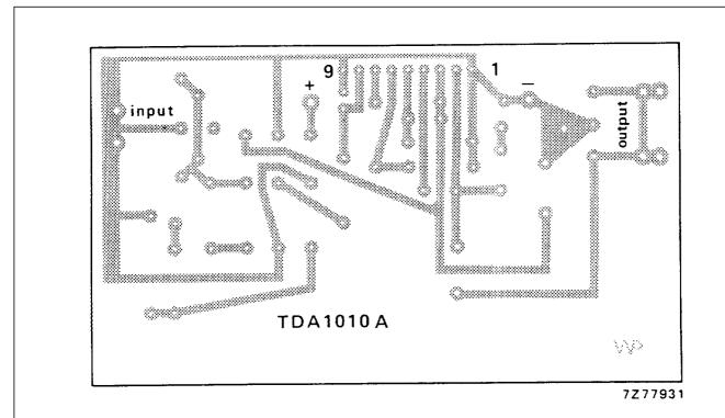
Fig.10 Track side of printed-circuit board used for the circuit of Fig.9; p.c. board dimensions 92 mm  $\times$  52 mm.
