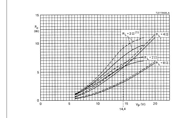
Fig.4 Output power of the circuit of Fig.3 as a function of the supply voltage with the load impedance as a parameter; typical values. Solid lines indicate the power across the load, dashed lines that available at pin 2 of the TDA1010.  $R_L = 2 \Omega^{(1)}$  has been measured with an additional 220  $\Omega$  bootstrap resistor between pins 3 and 4. Measurements were made at f = 1 kHz,  $d_{tot} = 10\%$ ,  $T_{amb} = 25$  °C.
