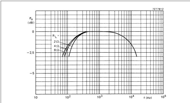
Fig.6 Frequency characteristics of the circuit of Fig.3 for three values of load impedance; typical values.  $P_0$  relative to 0 dB = 1 W;  $V_P$  = 14,4 V.
