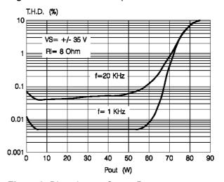
Figure 6: Distortion vs. Output Power
