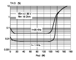
Figure 27: Distortion vs. Output Power
