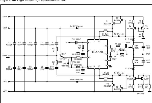
Figure 18: High Efficiency Application Circuit
