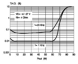
Figure 8: Distortion vs. Frequency
