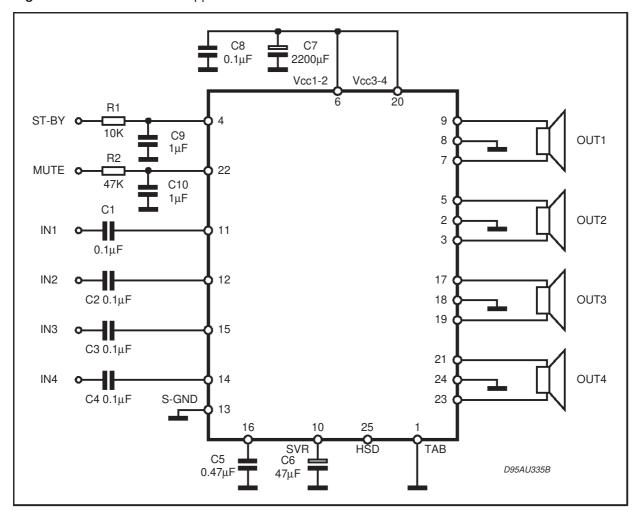
Figure 1: Standard Test and Application Circuit
