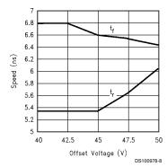
FIGURE 7. Speed vs Offset
