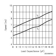
FIGURE 8. Speed vs Load Capacitance
