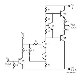
FIGURE 1. Simplified Schematic Diagram (One Channel)
