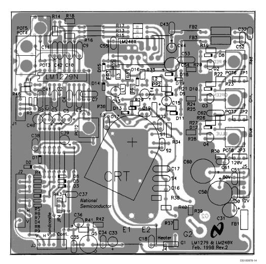
FIGURE 11. LM1279/240X Demo Board Layout
