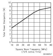
FIGURE 6. Power Dissipation vs Frequency
