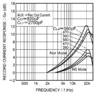
Fig. 23 Recording current response vs. frequency
