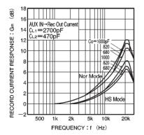
Fig. 21 Recording current response vs. frequency
