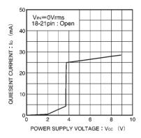
Fig. 6 Quiescent current vs. power supply voltage
