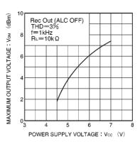
Fig. 8 Maximum output voltage vs. power supply voltage
