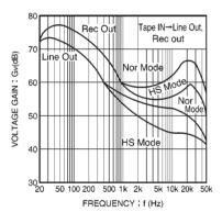
Fig. 18 Voltage gain vs. frequency
