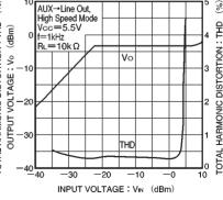
Fig. 14 Output voltage vs. input voltage
