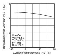
Fig. 9 Maximum output voltage vs. ambient temperature
