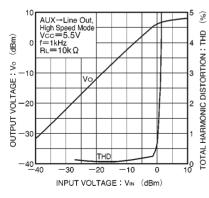
Fig. 12 Output voltage vs. input voltage
