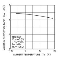
Fig. 10 Maximum output voltage vs. ambient temperature
