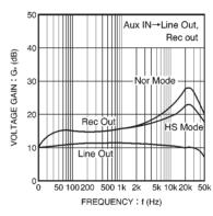
Fig. 19 Voltage gain vs. frequency
