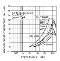
Fig. 22 Recording current response vs. frequency
