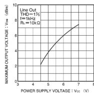
Fig. 7 Maximum output voltage vs. power supply voltage
