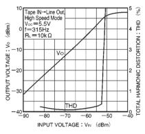
Fig. 11 Output voltage vs. input voltage
