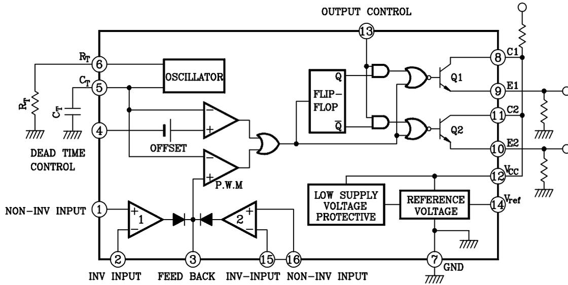
(Note) PIN ⑬ BECOMES SINGLE MODE AT "L" AND PUSH-PULL MODE AT "H"
