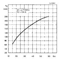
Figure 7: Distortion vs. Unloaded Q-factor of the Detector Coil.
