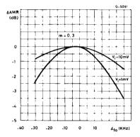
**Figure 4 :** Amplitude Modulation Rejection vs. Input Signal.
