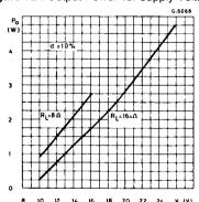
Figure 13: Power Dissipation vs. Supply Voltage (sine Wave operation).
