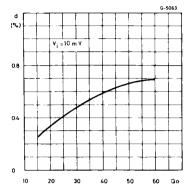
Figure 9 : Distortion vs. Tuning Frequency Change.
