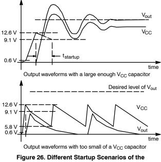
Circuits with Different V<sub>CC</sub> Capacitors
