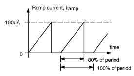
Figure 32. Internal Ramp Current Source
