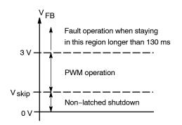
Figure 40. NCP1271 Operation Threshold
