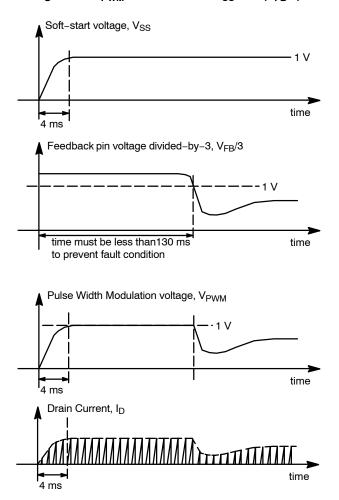
Figure 29. Soft-Start (Time = 0 at V<sub>CC</sub> = V<sub>CC(on)</sub>)
