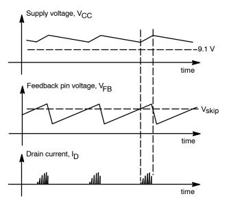
Figure 27. Timing Diagram of Standby Condition
