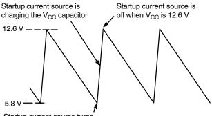
Startup current source turns on when  $V_{CC}$  reaches 5.8  $V_{CC}$
