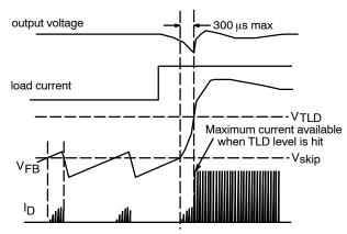
Figure 37. Transient Response from Standby
