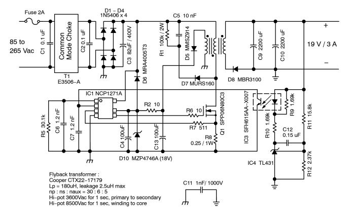
Figure 42. 57 W Example Circuit Using NCP1271
