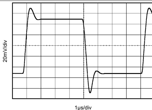
Figure 20. Large-Signal Step Response G = 1 , C_L = 1500\text{ pF} , V_S = \pm 15\text{ V}
