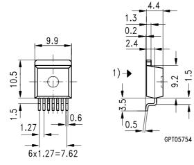
1) shear and punch direction no burrs this surface
