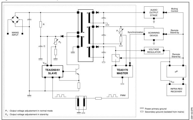
Figure 2 : Secondary Regulation (with optocoupler)
