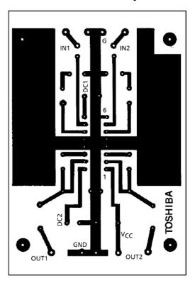
PCB: Epoxy glass 80mm × 60mm × 1.2mm
