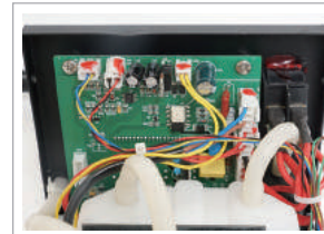
All in 1 PCB Metal screws fixed.
