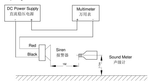
1. The red lead wire connect anode of DC power , The white lead wire connect cathode of DC power would make sound.
